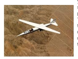
years. And in that time many designs have been tried, some proved more successful than others. The plane pictured is the AD-1, developed by NASA in the 1970's. The large wing on top actually swivels around as the plane flies, enabling it to become more sleek at higher speeds, reducing drag and increasing performance. It never did make it to production, but was flown successfully many times in testing.
